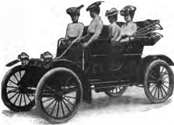
FIG. 86.—Haynes-Apperson Gasoline Surrey, one of the best-known makes of American motor carriage using wooden wheels.
